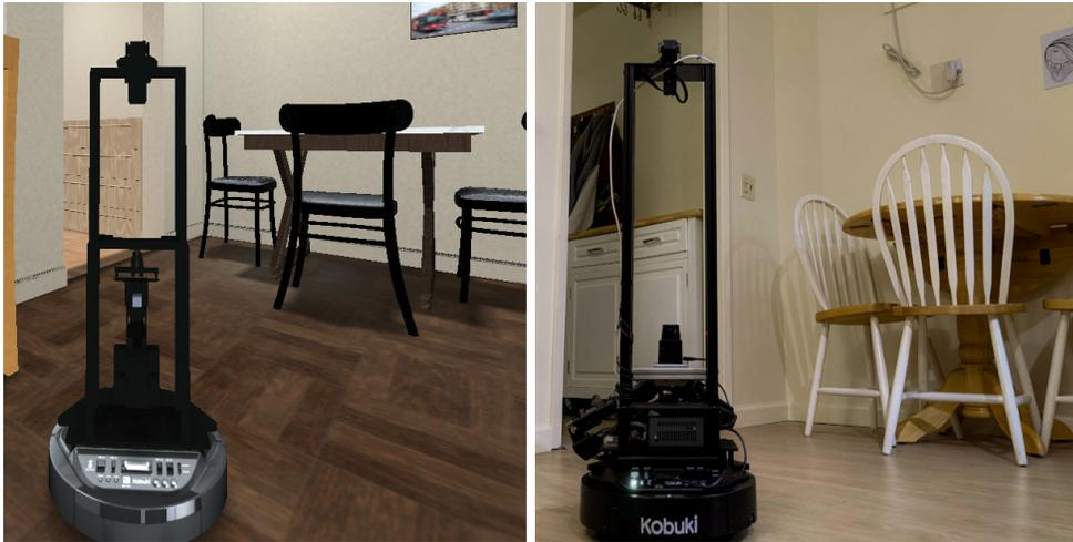
Figure 4.6: Robot navigating the real-world counterpart of the iGibson 1.0 scene `Rs_int`. The robot executes a policy trained in simulation with virtual LiDAR signals, without domain adaptation. The quality and realism of iGibson facilitates zero-shot policy transfer.
